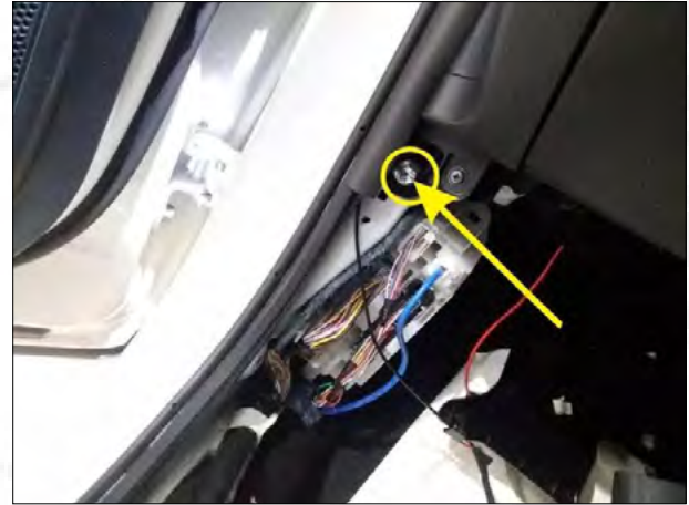
11. Connect the ground wire.
